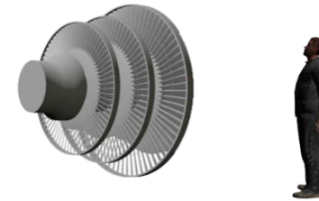
1 meter sCO 2 (300 MWe) (Brayton Cycle)
